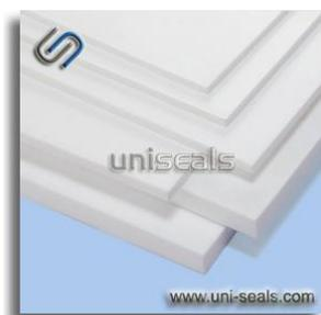
PTFE (polytetrafluoroethylene) has the best chemical resistance among known plastics. It also has good aging stability, electrical insulation, wear resistance, and extremely low friction coefficient. The unloaded operating temperature range is  $-180\sim+260^{\circ}\text{C}$ , and the dielectric strength is more than 10KV/mm.
